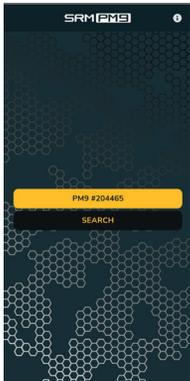
The SRM PM9 can be **connected to your smartphone** via Bluetooth®. If you are using Android, please make sure to give the app authorization for location access. This is required for the use of Bluetooth® LE. No information about your location is recorded.
