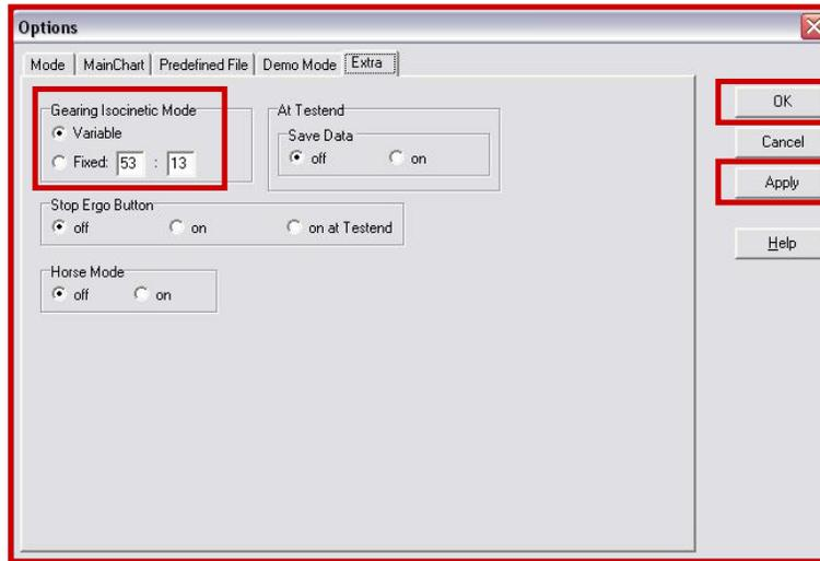
To enable an adjustment of cadence while maintaining a constant flymass angular velocity, or if you need a fast reaction of the brake, selected "Fixed" from the "Gearing Isokinetic Mode" section. In this mode, the controller will not adjust the brake when the gear selector is moved. The exact cadence can be modified by changing the chainring and cog tooth number in the boxes provided (and by shifting gears).
